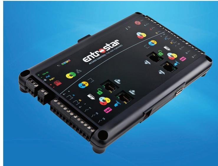
With innovative features for self-configuration and network discovery, EntroStar access control panels offer simple connection and interface to StarWatch systems.
