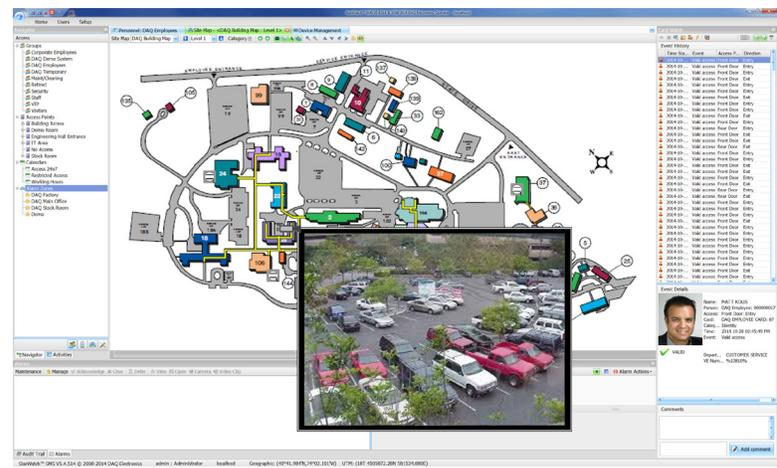
Fully integrated within the StarWatch SMS user interface, video display and management components are merged into interactive site maps and directly linked with alarms and events.
